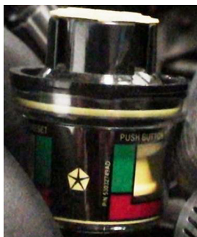
Figure 1. Air filter indicator from the 2007 Dodge Ram diesel truck. The yellow indicator reaches the red zone at 3.6 kPa differential pressure.
